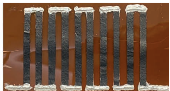
Fig.3. Digital photographs of the modules: (a) 10 p-type and (b) 5 p-n couple.
